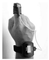
**CheckMeO2**: Press power button until display turns on, then insert index finger or thumb into sensor.
